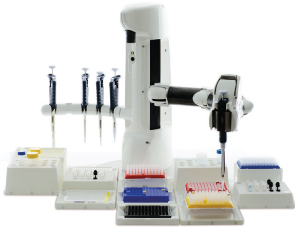
Figure 4: Andrew, the pipetting robot.
