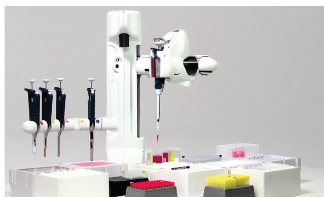
Figure 1: Andrew, the pipetting robot using conventional pipettes
