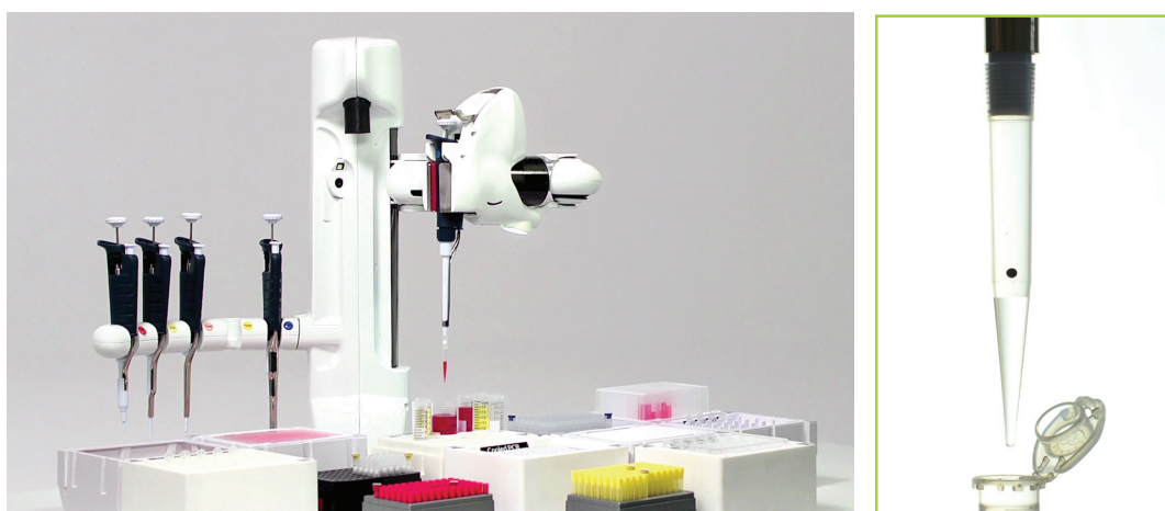
Figure 1: In-tip separation of beads from samples by the BeadTender method and the Andrew robot
