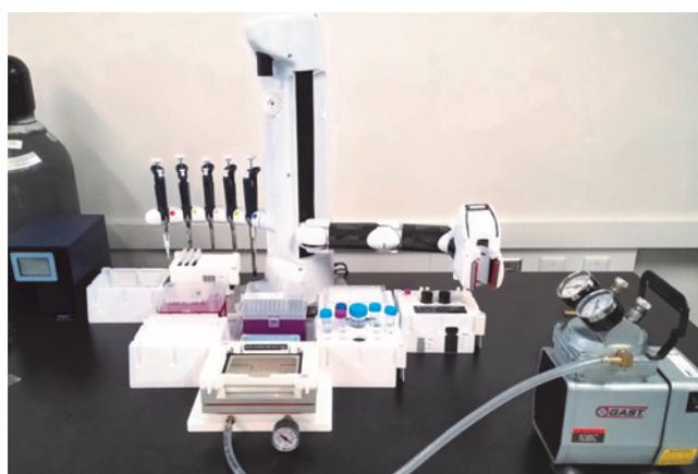
**Figure 2:** The workbench requirements of this automation protocol. Unique features include a heating/cooling feature, SPE cleanup component, released N-glycan kit component and vacuum manifold. Each block of the automation kit is modular allowing for adaptation to any protocol.
