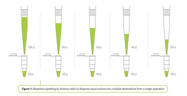
As the most flexible pipetting system, Andrew can change a pipette volume, insert and eject tips, aspirate, mix, dispense liquid, reverse pipette, forward pipette, deal with viscous solutions, create air gaps for eliminating dripping or tip touch for accuracy at low volumes, and adapt to the consumables on deck with artificial intelligence, from any source vessel type to any destination vessel type pre-determined by the users.
