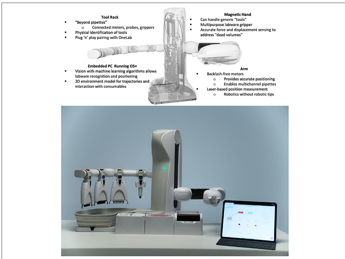
Figure 6. Disposition of Dominos, connected devices, and connected tools on Andrew+.
