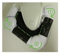
Fold the robotic arm till each portion is leaning against the foam block.
