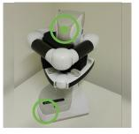
For moving the device, incline it gently backward by pushing onto its nose in order to grip the handle below the base.
