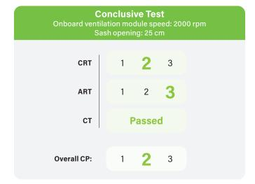
At 2000 rpm and with a sash opening of 25 cm, the airflow speed of the Andrew+ Pod is of 0.25m/s. This corresponds to an air volume flow of 222m<sup>3</sup>/h.
